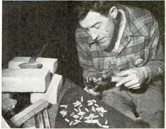
This hunter is molding his own bullets to reload his shells
